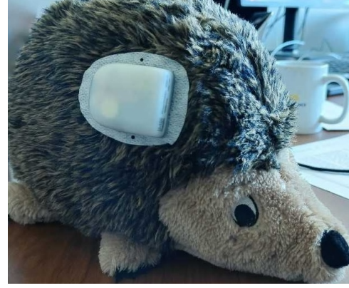
Figure 11. We attached an Omnipod DASH insulin pump to a stuffed animal and modified the OmniB LE pump driver to intentionally add, drop and modify insulin commands. Our driver security mechanism detected all manipulations.
